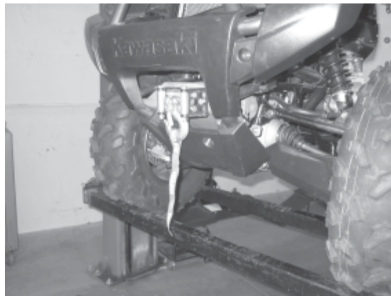
Figure 6 Install Winch and Roller Fairlead
